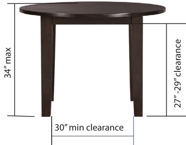
Accessible: 4 vertical legs on a round table top. Ensure that the clear width between legs is 30" minimum.
